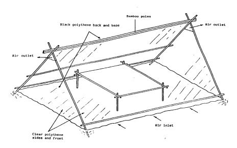
Figure 1: Typical tent solar dryer
