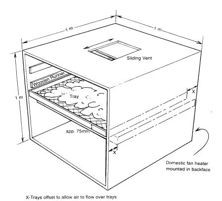
Figure 5: Small electric dryer. The air should follow a zigzag path.
